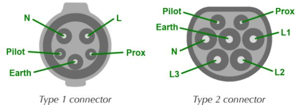
If only a single charger is used with a Type 2 connector, its AC supply should be connected between Neutral and L1. L2 and L3 are used where three chargers are present, for three phase charging.
