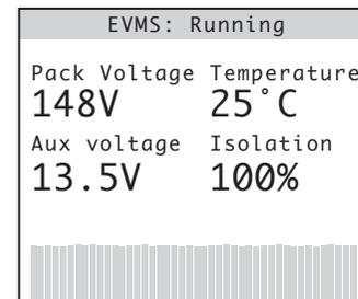
If no current sensor is present on the CAN bus, the EVMS is unable to show current or calculate power or state of charge, so a different page is shown with only pack voltage, temperature, aux voltage, isolation, and a bar graph of all individual cell voltages.
