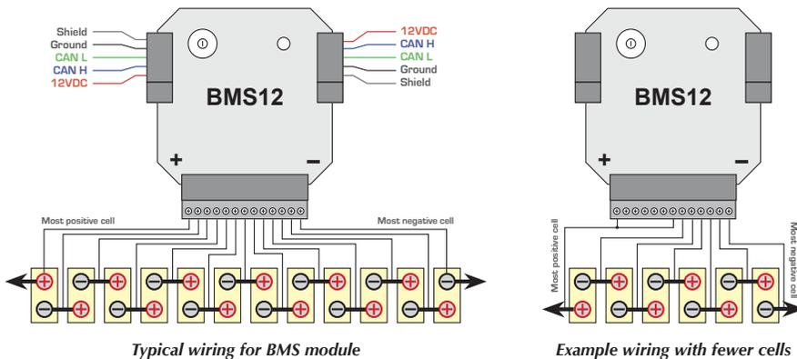
Each BMS module needs to be assigned a unique ID using the rotary selector on top, and the EVMS gets configured for how many cells it should expect at which BMS IDs.
