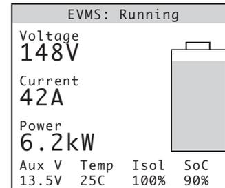
The main display, showing EVMS status at the top, instantaneous voltage, current, power, auxiliary battery voltage, temperature, isolation, and State of Charge (SoC).
