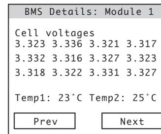
Detailed information for a single BMS module, showing voltage of each cell (to 3 decimal places) and two temperatures if available. Orange bars beneath the voltages indicate if cell shunts are currently on.
