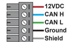
*Note that while connectors into most devices go screw side up, due to the orientation of the internal circuit board in the EVMS3, its CAN plugs are inserted with screw side down.*
