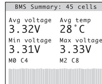
BMS summary page, showing the total number of cells being monitored, the average voltage per cell, the average of any BMS temperature sensors, and the voltage and location of both the lowest and highest cells. *M* is Module ID, *C* is the cell number.
