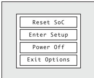
You can bring up the options menu by touching and holding for 1 second. From here you can do a manual reset of the State of Charge (back to 100%), enter the Setup mode, switch the display off, or command the BMS16 to turn off.
