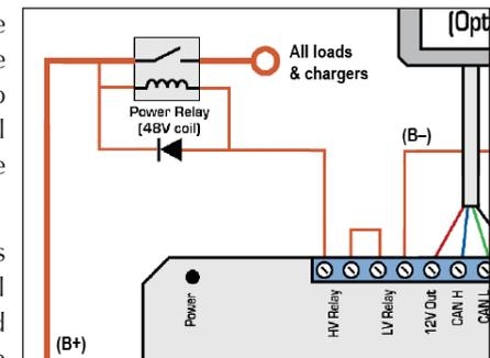
Note that in this configuration, if the BMS opens the main contactor due to an under-voltage cell for example, the battery pack will also be isolated from any charging sources so will be unable to charge (and correct the under-voltage condition) until the system is reset manually. For this reason it is important in this case that BMS intervention is an exceptional circumstance, and under normal operation chargers and loads will not cause any cells to exceed safe range.
