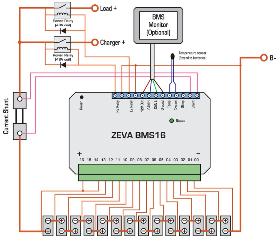
Relay outputs are floating / isolated, and have a maximum rating of 60V and 1.3A continuous. Be sure to include a flyback diode (if not built in to the relay/contactor) to suppress inductive voltage spikes from switching the relay coil. In installations with a single “battery enable” relay, the LV and HV relays may be wired in series such that either an over-voltage or under-voltage condition will open the relay to isolate the battery pack.
