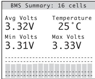
The BMS Summary page shows the average, minimum and maximum cell voltages, and the temperature sensor, plus a bar graph overview of all cells across the bottom.
