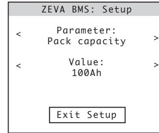
If you choose Enter Setup, the Monitor can be used to modify settings for the BMS16. The top row selects the parameter, and the bottom row adjusts the value, in both cases by touching the left or right arrows on each side. Once finished, touch Exit Setup and the new parameters will be transmitted to the BMS16.
