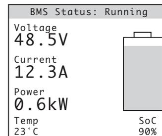
The BMS Status page is the standard display when the system is running, showing pack voltage, current, power, temperature, battery state of charge. This will only be shown if a current sensor is present.
