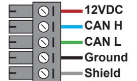
Wire gauge around 20-24AWG is recommended for appropriate current rating and mechanical strength. For best noise immunity in high EMI environments, shielded twisted pair cable is recommended, with two conductor pairs – one pair for CAN signals, and one pair for bus power. The shield can be connected to the Ground terminal at the BMS. We use and recommend Belden 8723 wire, or equivalent.
