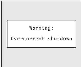
If the BMS detects an error, this warning page will be displayed. In most cases, the error can be acknowledged/reset by tapping the screen.
