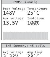
If no current sensor is present on the CAN bus, the EVMS is unable to show current or calculate power or state of charge, so a different page is shown with only pack voltage, temperature, aux voltage, isolation, and a bar graph of all individual cell voltages.
