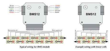
Each BMS module needs to be assigned a unique ID using the rotary selector on top, and the EVMS gets configured for how many cells it should expect at which BMS IDs.
