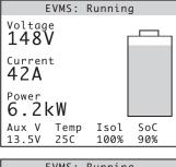
The main display, showing EVMS status at the top, instantaneous voltage, current, power, auxiliary battery voltage, temperature, isolation, and State of Charge (SoC).
