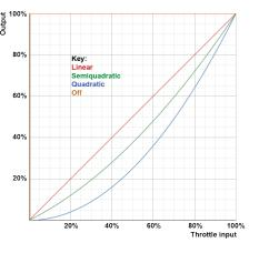
The default setting of Linear for both speed and torque is suitable for most series DC motors, giving a familiar driving experience. For permanent magnet motors, usually semiquadratic torque control works well, with speed control either Off or in Linear mode. Speed only control is not normally suited to traction applications (cars/bikes) but can be useful for aircraft or boats.
