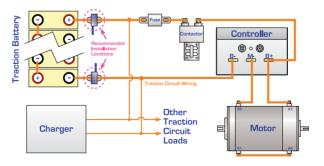
The flow of conventional current (+ve to -ve) should go from the back to the front of the current sensor – that is, the side with the mounting bracket should be oriented towards the positive terminal.
