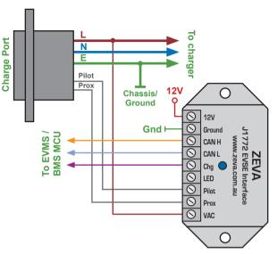
The LED terminal will mirror the behaviour of the LED on the device, optionally used for powering a remote LED in a more visible location. The output has a 5mA current limit (no series resistor required).
