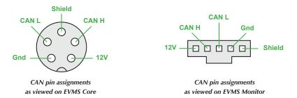
CAN buses work best when wired as a single daisy chain of devices, with 1200hm termination resistors at each end to prevent signal reflection. Most ZEVA CAN-enabled devices have dual CAN ports for easy daisy-chaining. The order of devices is unimportant - usually the shortest path between devices is best.
