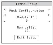
The Setup mode has three rows. The top row toggles between the General Settings and the Pack Configuration sections. Tap the arrows either side to nagivate between these. In the General Settings page, the second row selects the parameter to be modified, and the third row modifies the parameter itself. The Exit Setup button will distribute new settings to all devices on the network then return to normal operation.
