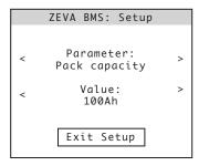
If you choose Enter Setup, the Monitor can be used to modify settings for the BMS16. The top row selects the parameter, and the bottom row adjusts the value, in both cases by touching the left or right arrows on each side. Once finished, touch Exit Setup and the new parameters will be transmitted to the BMS16.
