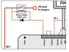
charge (and correct the under-voltage condition) until the system is reset manually. For this reason it is important in this case that BMS intervention is an exceptional circumstance, and under normal operation chargers and loads will not cause any cells to exceed safe range.
