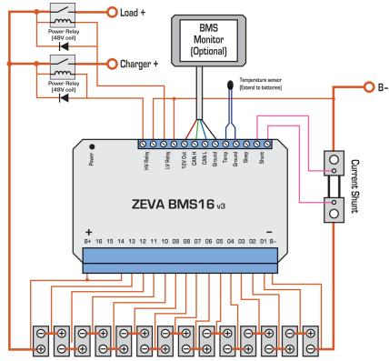
Relay outputs are floating / isolated, and have a maximum rating of 70V and 1A continuous. In installations with a single "battery enable" relay, the LV and HV relays may be wired in series such that either an over-voltage or under-voltage condition will open the relay to isolate the battery pack as shown on the following page.
