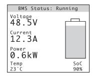
The BMS Status page is the standard display when the system is running, showing pack voltage, current, power, temperature, battery state of charge. This will only be shown if a current sensor is present.
