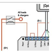
Note that in this configuration, if the BMS opens the main contactor due to an under-voltage cell for example, the battery pack will also be isolated from any charging sources so will be unable to charge (and correct the undervoltage condition) until the system is reset manually. For
