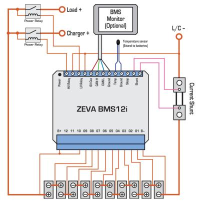
Relay outputs are floating / isolated, and have a maximum rating of 60V and 1A continuous. In installations with a single "battery enable" relay, the LV and HV relays may be wired in series such that either an over-voltage or under-voltage condition will open the relay to isolate the battery pack as shown on the following page.
