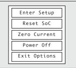
You can bring up the options menu by touching and holding for 1 second. From here you can do a manual reset of the State of Charge (back to 100%), enter the Setup mode, switch the display off, or command the BMS12i to turn off.
